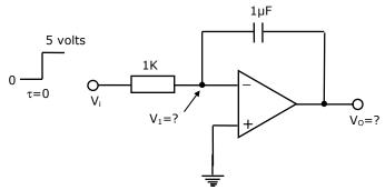
7. In figure, the operational amplifiers are ideal and their output can swing between -15 and +15 volts. Sketch on same diagram, the waveform of voltages  $V_1$  and  $V_2$  as a function of time. You must give the values of important parameters of this sketch.
