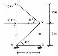
A pin jointed truss is loaded as shown in the above figure match List I with list II and select the correct answer:
