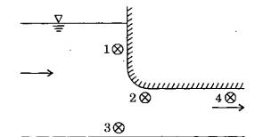
A sluice inlet in a dam with streamlined entrance is shown in figure. If cavitation is expected to occur, it will first appear at the point
