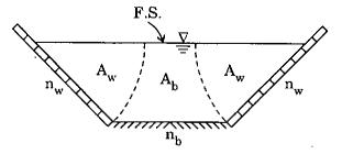
The two sides of a trapezoidal channel are lined with cement plaster,  $n_w = 0.012$ , while the earthen bed has  $n_b = 0.025$ , the area is divided into three parts as in the figure.
