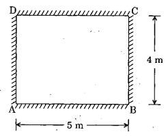
The RC slab, simply supported on all edges as in above figure, is subjected to a total UDL of 12 kN/m<sup>2</sup>. The maximum shear force/unit length along the edge BC' is
