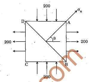
A square element is subjected to principal stresses in  $N/mm^2$  as in figure. The intensity of normal stress  $\sigma_n$  on plane BD is
