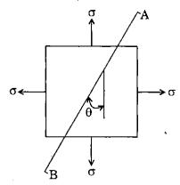
A point in two-dimensional stress state subjected to biaxial stress is shown in figure. What is the normal stress acting on the plane AB?
