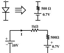
Now applying KVL for Linear circuit
