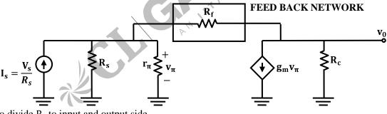
To divide R<sub>f</sub> to input and output side
