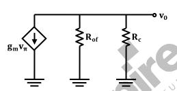
$$A = \frac{V_0}{I_S} = -\frac{g_m(R_f||R_c)v_{\pi}}{\frac{v_{\pi}}{(R_s||R_{if}||r_{\pi})}} = -g_m(R_{of}||R_c)(R_s||R_{if}||r_{\pi})$$
