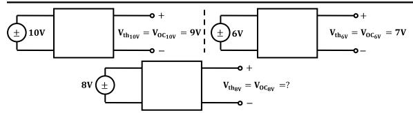
Since, two port network is linear non reciprocal, output (at port 2) can be expressed as a linear function of input.
