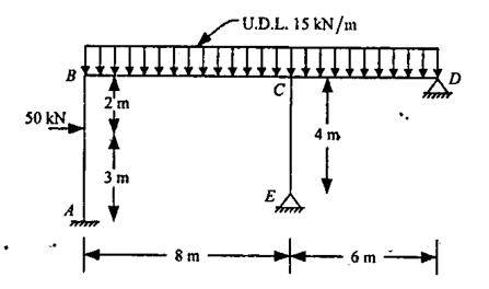
Analyse the rigid frame shown in the above figure by moment distribution method, taking flexural rigidity EI to be uniform for all members. 20
