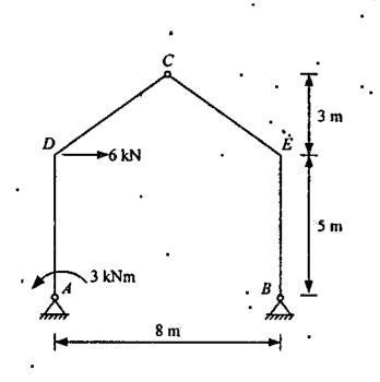
Find all the support reactions and draw BM diagram for the frame shown above. Frame has hinged supports at A & B and internal hinge at C.
