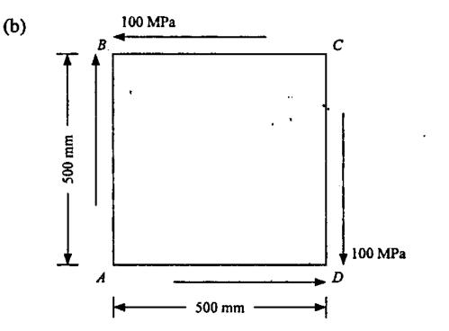
A square plate of side 500 mm is subjected to pure shear of intensity 100 MPa as shown in the above figure. Young's modulus of the material is  $2 \times 10^5$  MPa and Poisson's ratio is 0.2. Find the principal stresses, their directions and the change in lengths of the diagonals of the plate. 10
