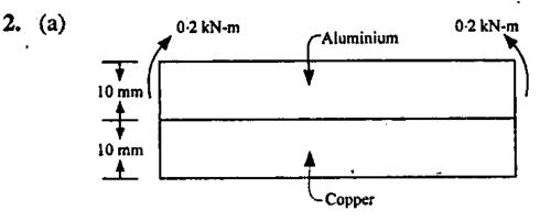
A strip of copper 40 mm wide and 10 mm thick is bonded with another strip of aluminium of same size to form a bimetallic strip of 40 mm × 20 mm. The strip is subjected to a pure bending moment of 0.2 kN-m as shown in the above figure. Calculate the radius of curvature of the strip and the maximum tensile and compressive stresses.  $E_c = 1 \times 10^5$  MPa,  $E_{al} = 0.6 \times 10^5$  MPa. 20
