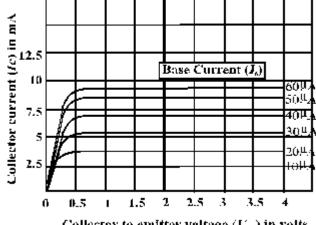
Collector to emitter voltage  $(\Gamma_{cz})$  in volts
