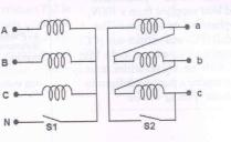
The star-delta transformer shown above is excited on the star side with a balanced, 4-wire, 3-phase, sinusoidal voltage supply of rated magnitude. The transformer is under no load condition.
