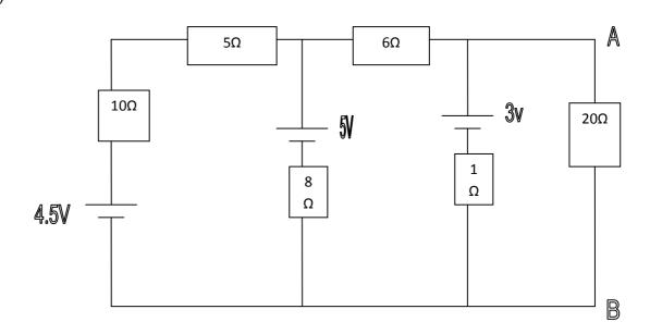
Find out the voltage  $V_{ab}$  by applying Norton's theorem.
