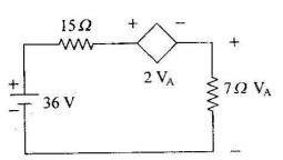
The power dissipated in the controlled source of the network shown above is
