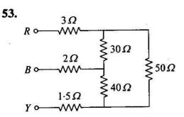
A 3-phase distribution network is as shown above. The resistance across the terminals *RB*, *BY* and *RY* are
