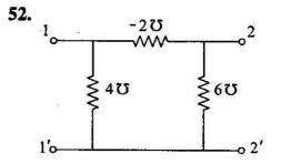
For the two port network as shown above, the parameters  $h_{11}$  and  $h_{21}$  are
