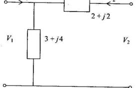
The Z-parameter matrix of the two-port network as shown above is
