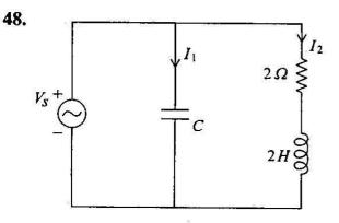
In the network shown above  $V_s = 4 \cos 2t$ . The value of C is so chosen that the circuit impedance is maximum. Then  $I_1$  leads  $I_2$  by
