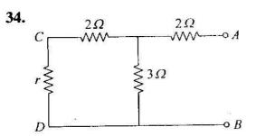
For the circuit shown above the value of r connected between C and D is such that the equivalent resistance of the circuit by looking into circuit through terminals A and B is r only. Then the value of r is
