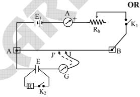
Close key  $K_1$  keeping key  $K_2$  open. Find the point (say J) on the wire AB such that on pressing the jockey on the wire at J, the galvanometer gives no deflection. At this stage, the potential difference across A and J is equal to the e.m.f. (E) of the cell.
