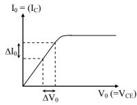
Output resistance =  $\frac{\Delta V_0}{\Delta I_0}$
