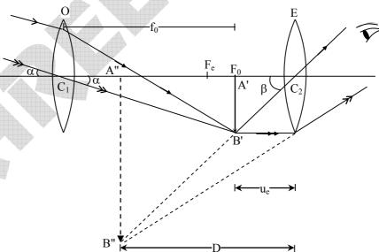
Magnifying power of an astronomical telescope is defined as the ratio of the angle subtended by the final image at the eye to the angle subtended by the object at the eye.
