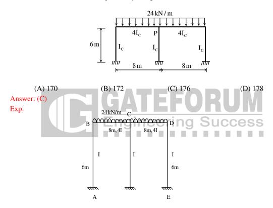
Axis of symmetry is passing through a column; hence it can be treated as
